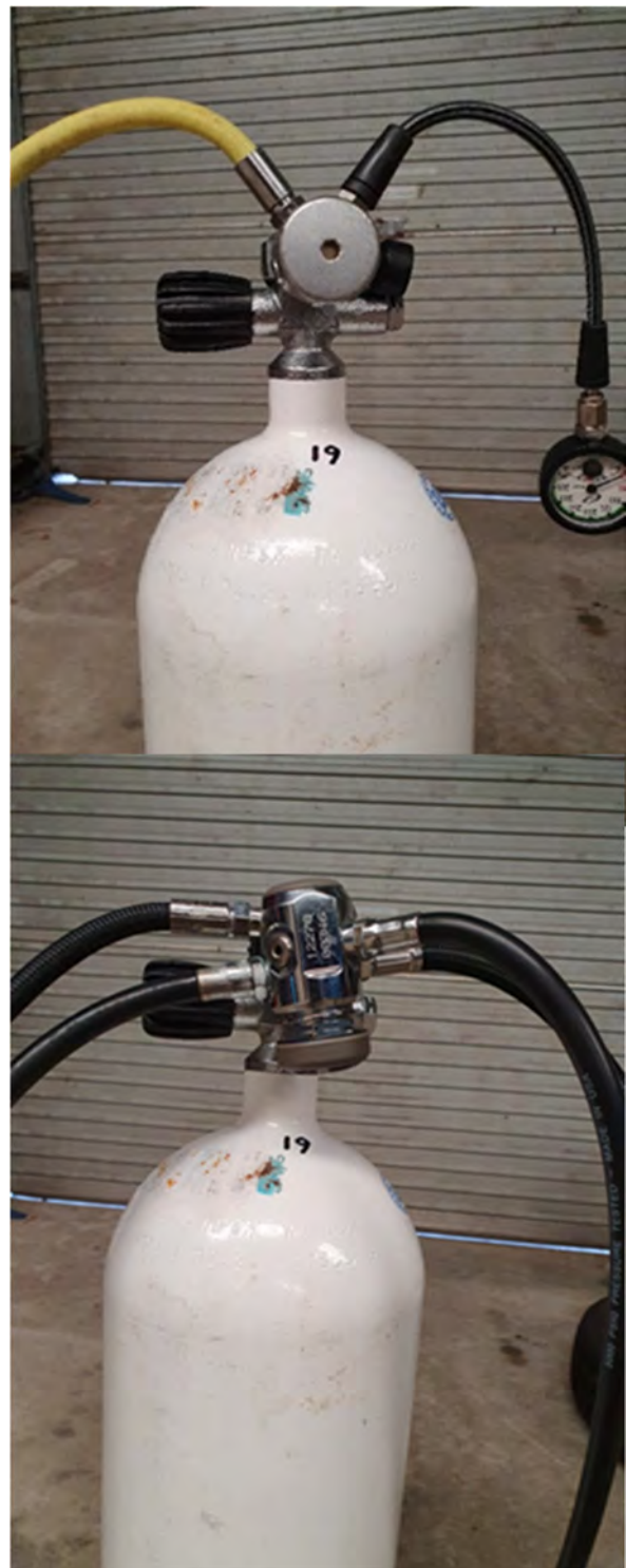
Figure 5. The regulator top image has the hoses directed upwards. The regulator bottom image has the hoses directed as horizontally as possible. Nobody says the first stage body has to be vertical. Sure it looks nicer but unexposed hoses are better.
