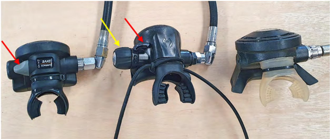
Figure 1. Three regulator second stages showing different air flow adjustment systems. The red arrows show venturi adjustment knobs and lever, while the yellow arrow shows a second stage valve adjustment knob. The regulator on the right has no adjustments.
