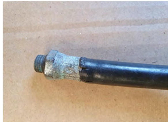
Figure 4. Examples of damage to a second stage LP regulator hose that should have been replaced a long time ago!
