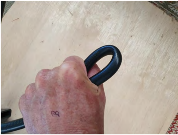
Figure 2. A tightly bent second stage LP hose. The bend is sufficient to completely stop the flow. If not, squeeze harder.
